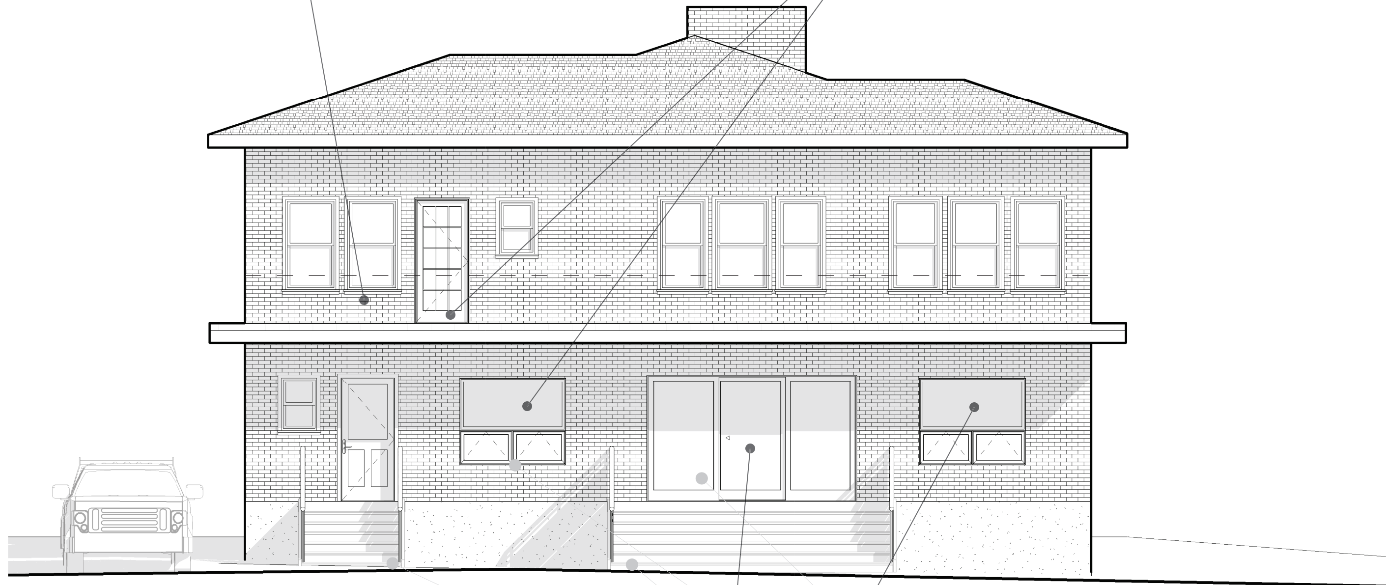
BRICK DISPLACEMENT @ CANOPY
